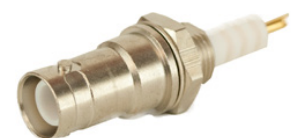
SHV - Shielded High Voltage Offers the most protection and a shield that can be grounded but more expensive and hardest to wire.
